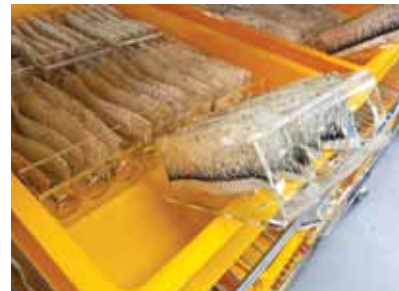
From left: The Wolbachia mosquito factory is highly automated. This is a machine for separating male and female pupae. Photo: Huang Ning Xin; Eggs of Wolbachia -infected mosquitoes. Photo: Dr Ngo Kang Min.
